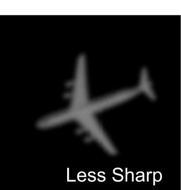
2D Gaussian sampling kernel used to apply appropriate blurring to rendered CAD model.
